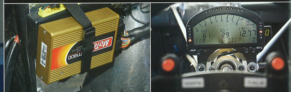
Below: full data logging from Motec ECU while PI dash cuts down on unnecessary gauges
