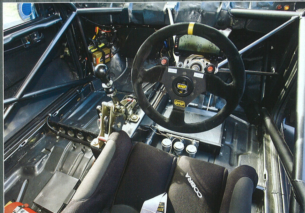
Below: full data logging from Motec ECU while PI dash cuts down on unnecessary gauges
