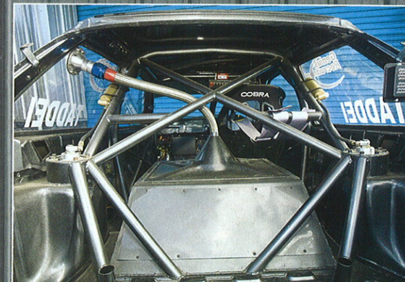
DJM designed and built the cage and fuel cell housing
